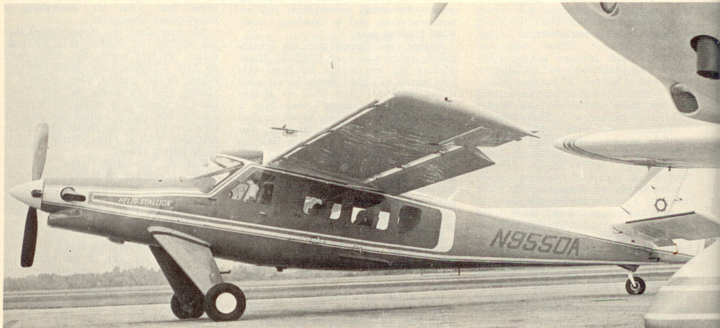
The vane at the left of the Turbo Stallion's wing activates a stick-force augmentation system (SFAS). Note the long flaps (72 percent of the trailing-edge span).
